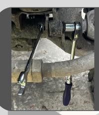
You need a closed-end wrench, a ratchet drive & socket. Place the closed-end wrench and socket on the nut and bolt. (Left loose)
