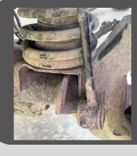
Once you pull out the bolt make sure to put the nut back on the bolt so don't lose it.
