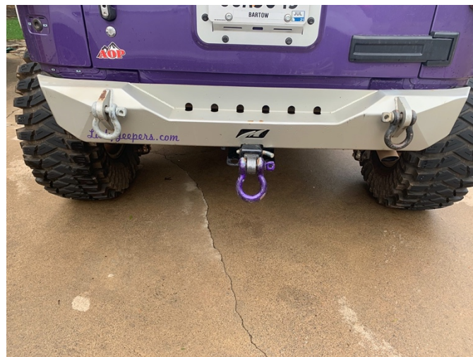
(Secure the strap to a safe recovery point on the rear of the tow vehicle)
