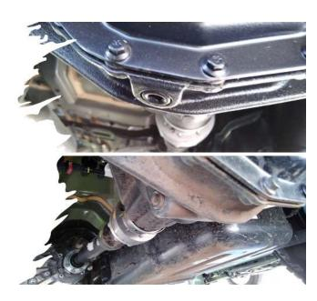
You will need to look for the differential drain plug on the differential housing. Locate the drain plug and you can determine the axle.
