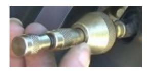
Detach the tool - unscrew the center piece to the left until the tool is no longer attached and is off the tire.
