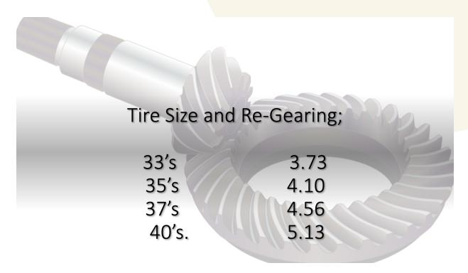
The tire size and gearing go hand in hand. This is a minimum requirement. If you are going to spend the money to re-gear do not re-gear to the minimum requirement! Go one gear ratio deeper (or larger number). This chart shows the absolute minimum gear to have in your Jeep when you go to the new tire size. If you have stock 3.73 gears in your Jeep, you can put a 33" tire on without regearing. If you have a stock 4.10 gear, you can put a 35" tire on without re-gearing.
