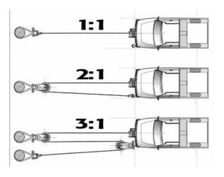
The ratios of using multiple snatch blocks as outlined on the previous page. You can replace trees with another vehicle as well and use multiple positions if you have a heavy vehicle or are very stuck to ease the load on the winch or take pressure off the anchor vehicle as well.
