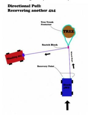
NOTE: You can use another Vehicle or a Tree for the anchor point on the recovery. So you would run the Winch Hook to the D-ring on the front or back of another vehicle or to another tree saver strap with a D-ring on your anchor tree.
