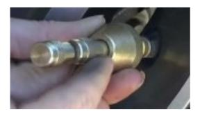
Attach the tool to the valve stem. Hold forward on the air release (the big round piece) line up the threads and screw the center piece of the tool to the right until snug.
