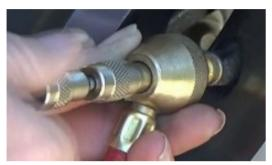
Tighten the plunger - Push the plunger piece in and twisting to the left until it no longer wants to twist and the plunger starts to push out against you. Then pull the plunger out. This slides the long plunger out from the end you were twisting.
