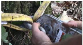
Close your snatch block by twisting back and run the open end of the snatch block through the pin of the D-ring to secure it to the tree strap and anchor.
