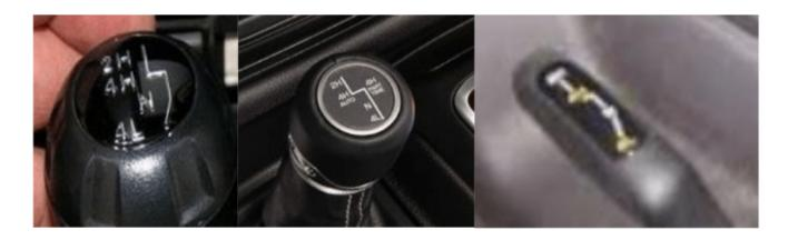
Though as you can see, the shifters in different Jeeps can vary you will notice that all the shifters have a 2H setting, a 4H setting, a Neutral and a 4 Low. On majority of shifters your 2H or 2 Wheel Drive setting will at the very top left setting. The 4H or 4 Wheel Drive High will be shifting straight down. Exception: The newer generations have a 4H all time and 4H part time setting. You will want to shift down and over to the right to shift into the 4 Wheel Drive Part time setting.
