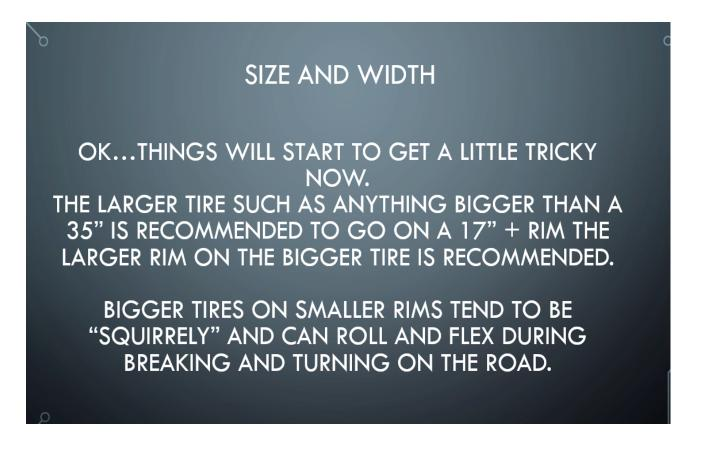
Moving into putting the tire and wheel together it is about the size and width. The larger tire, such as any tire that is going to be a 35 inch or bigger is recommended to go on a 17 inch wheel or larger.
