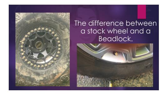
When mounting the non-beadlock on the right, it actually mounted so that the rubber of the tire is put underneath the lip of this wheel and then they go ahead and inflate it with air all the way. What is holding this together and creating the seal is the actual air pressure.
