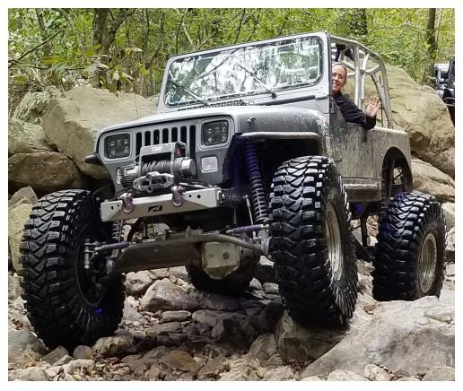
In this photo I have a high profile fender upfront and fender delete in rear, to allow room for this 42" tire. The bigger the tire the more lift you need or the more room in the wheel well you have to create to give the tire room to move. This of course is just one piece in the larger overview build scale.
