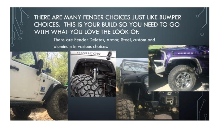
A quick re-cap. There are fender deletes, which is going to be like this white JKU here second from the left. It is the one where there is no fender, and means you have nothing sticking out from the Jeep to impede with your tire. Then there is steel which is normally black, on the far left white JKU. You can go a complete custom route like the CJ5 second from right. You also have the choice of aluminum, far right.
