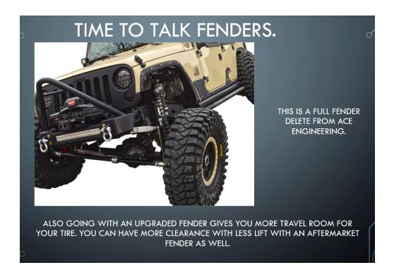
The photo above shows one common type of fender upgrade. This is the full fender delete. The pictured fender delete is from ace to engineering.
