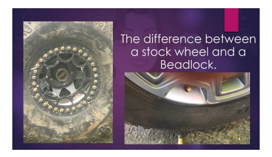
When mounting the non-beadlock on the right, it actually mounted so that the rubber of the tire is put underneath the lip of this wheel and then they go ahead and inflate it with air all the way.
